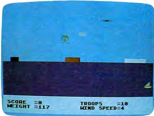
Atari "Paratrooper" uses player/missile graphics, a display list interrupt, and machine language to smooth out the action.
