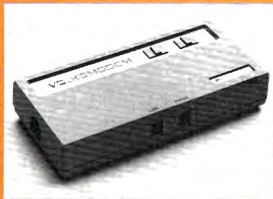
Direct-connect modems, such as this Volksmodem, plug right into the modular phone jack and are generally more reliable than acoustic modems.
