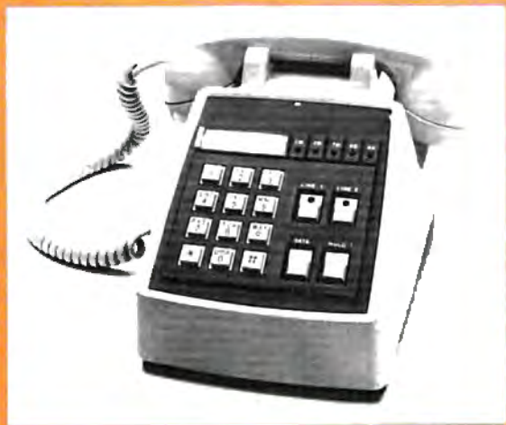
Code-A-Phone's Tel-A-Modem 212A is a telephone with a built-in modem and two phone lines for simultaneous voice and data transmissions.
