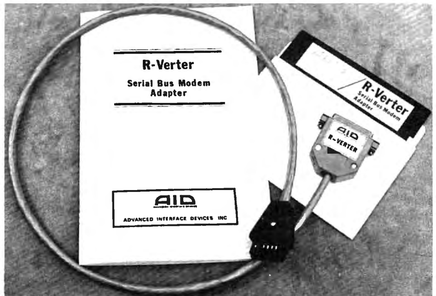
The R-Verter allows most modems and other RS-232C devices to be used directly with Atari computers without using the Atari 850 Interface Module.
