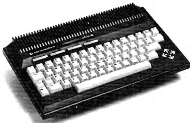
Commodore's new Plus/4 computer—a revised version of the 264 shown by Commodore last January—has four programmable function keys and four separate cursor keys.
