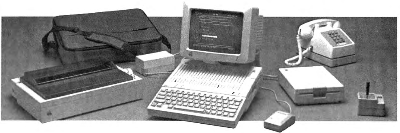
The Apple IIc, with optional 9-inch monitor, Scribe thermal transfer printer, AppleMouse II, external disk drive, joystick, modem, and carrying case.
