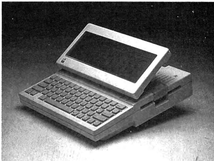
By September, Apple promises this flat LCD screen, which fits on top of the main IIc unit and has full 80-character by 24-line display.
