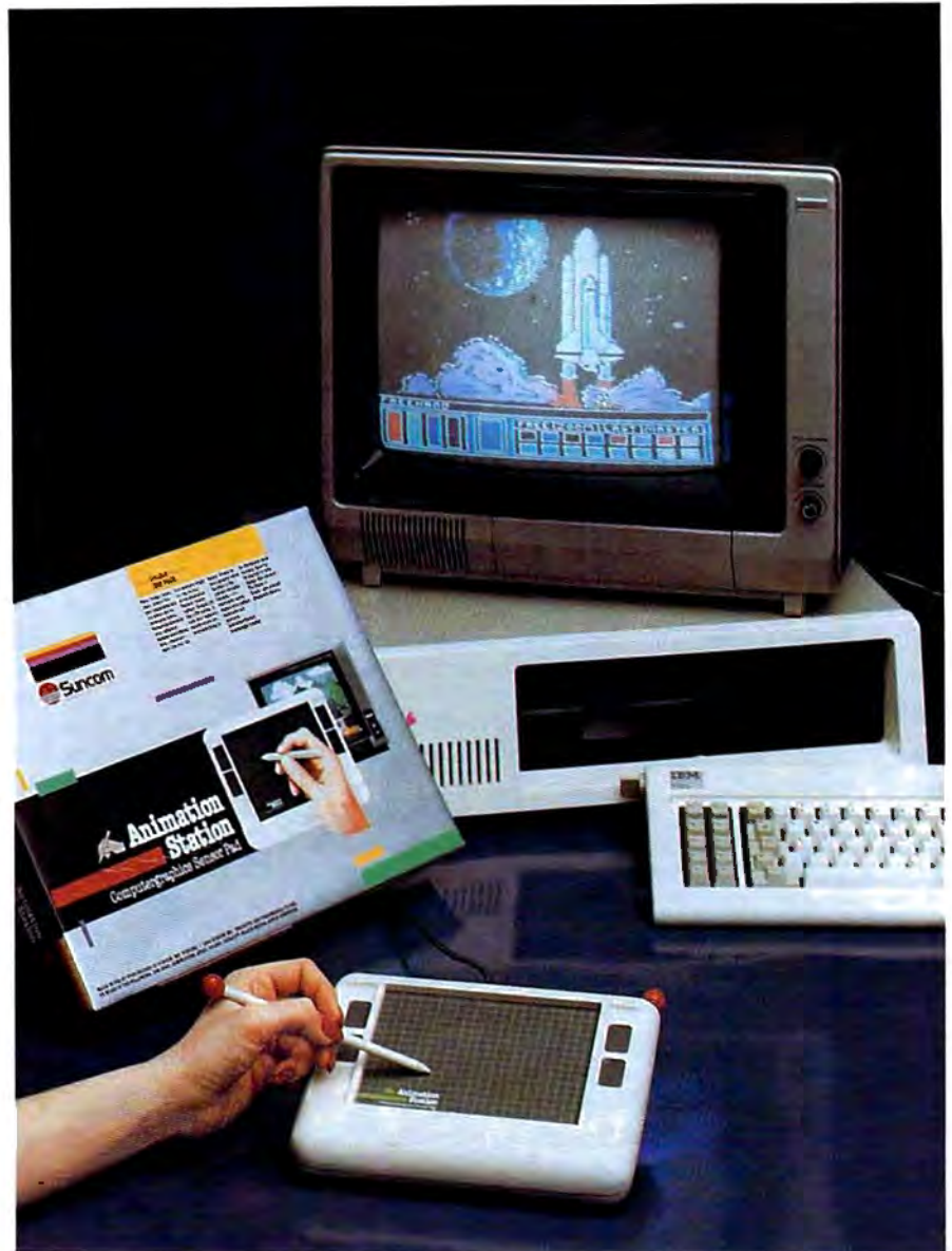
Animation Station, a graphics tablet designed by Suncom, offers a number of colors and textures for drawings like this.
