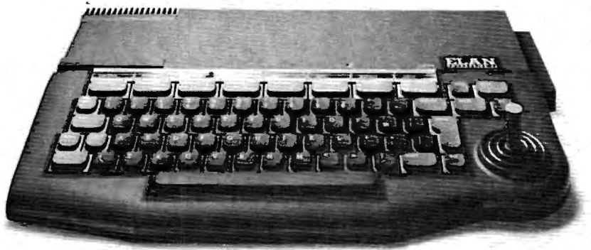
The sleek Elan Enterprise from Britain. Notice the built-in joystick. Two more sticks can also be plugged in.
