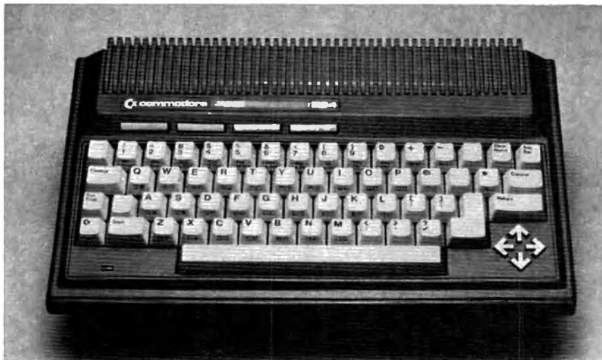
The Commodore 264. Note the unusual arrow-shaped cursor keys. The Commodore 364V is similar, but has a numeric keypad to the right of the keyboard.
