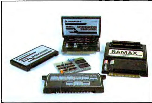
Memory expanders give you additional work room within your computer. Expanders range from simple memory chips to complicated boards with cartridge slots and reset buttons.
