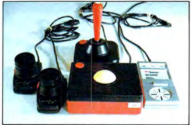
Game controllers come in a variety of styles, each of which has a different "feel." Shown here are paddles, a joystick, a trackball, and a pressure-sensitive controller.
