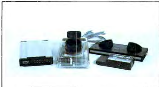
Modems let your computer exchange information with other computers via telephone lines. Direct connect modems plug directly into the phone line. With an acoustic modem, the telephone handset fits into a pair of soft cups.
