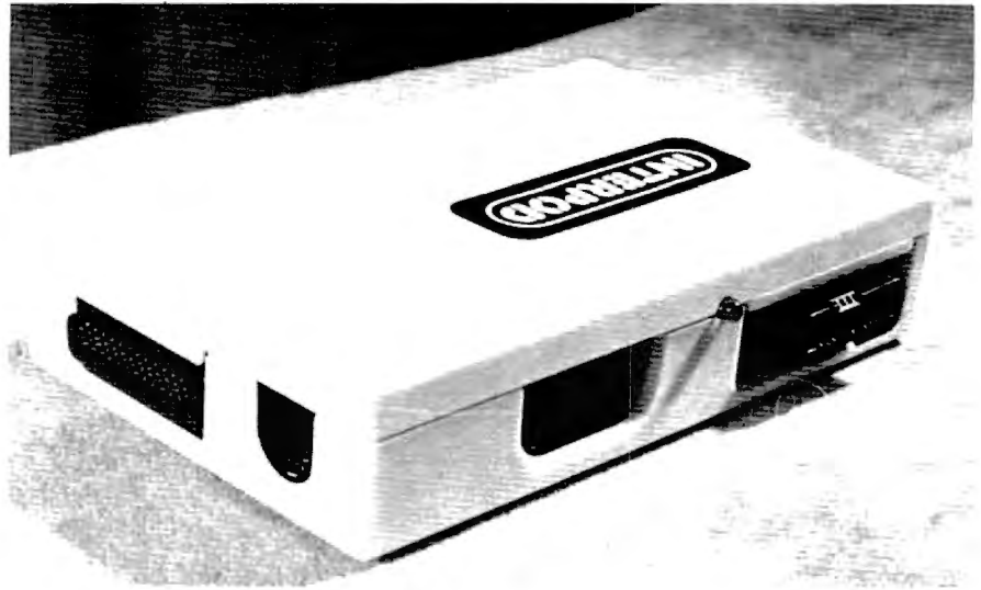
Interpod module contains both an IEEE port and RS-232 port to support output. It also has a power supply connection and two serial attachments for the VIC/64 mating cable and a spare outlet for a serial unit such as a 1541 disk drive.
