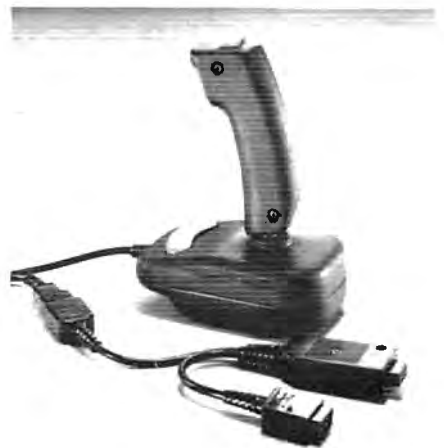
The TI version of the Competition Pro 3000 joystick includes an adapter for the TI-99/4A computer.
