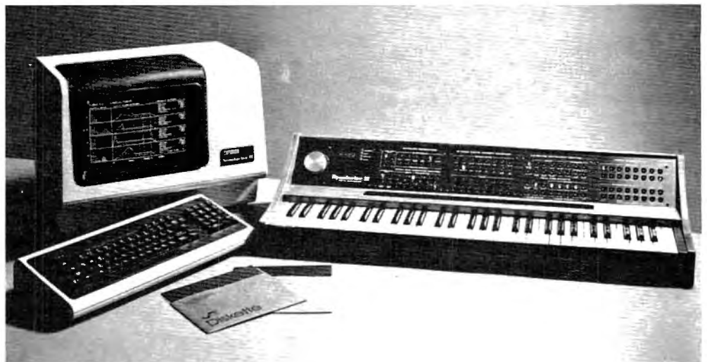
A video display of waveforms and a computer keyboard accompany New England Digital's Synclavier II.
