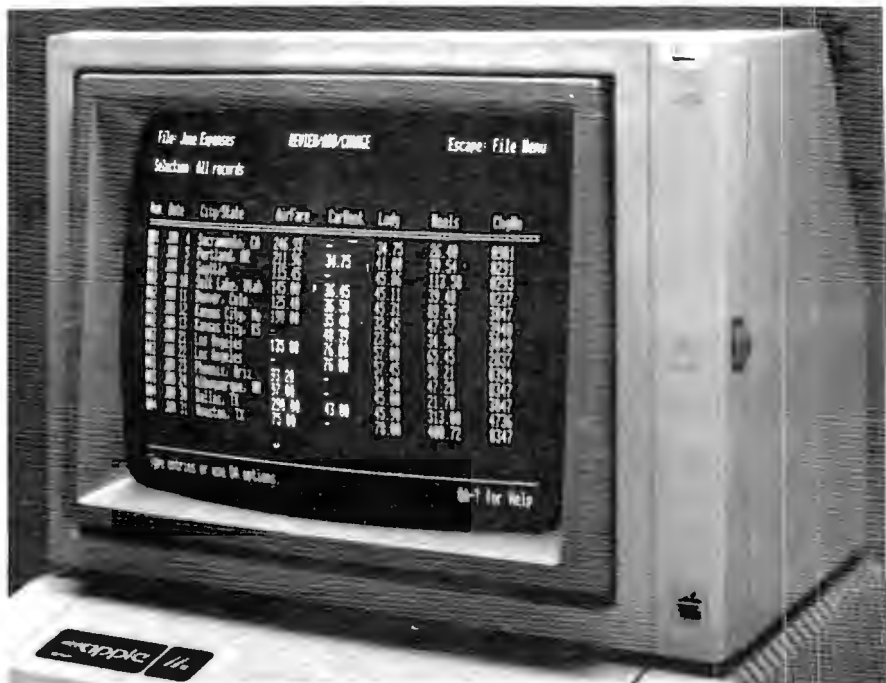
Apple's new 12-inch monochrome monitor includes a tilt mechanism to adjust the angle of the screen.
