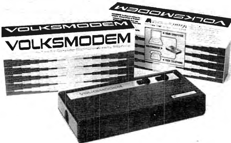
Anchor Automation's Volksmodem can interface with most personal computers via a separate cable. It is a direct-connect modem.
