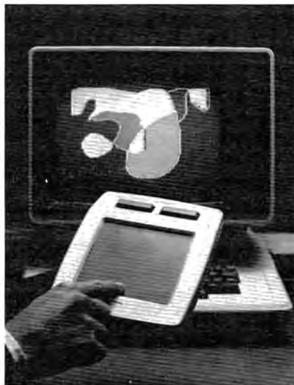
The Koalapad Touch Tablet can be used for drawing or as an auxiliary keyboard.
