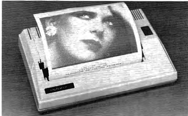
Alphacom 81 is an 80-column thermal printer with graphics capabilities.
