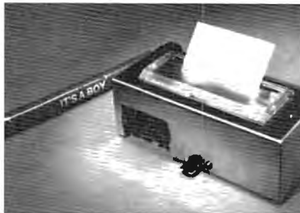
Panasonic's EUY-3T miniature thermal printer.
