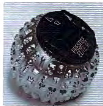
Close-up of an IBM Selectric ball. Some electronic typewriters can also function as computer printers with the proper interface.
