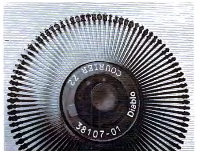
Some letter-quality printers are called “daisy wheel” printers because they use a print head shaped like a daisy with letters on the ends of the petals.
