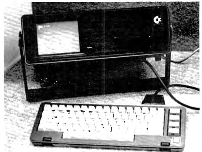
Commodore's prototype SX-100 with built-in color monitor and twin disk drives. Note the detachable lid/keyboard and carrying handle.
