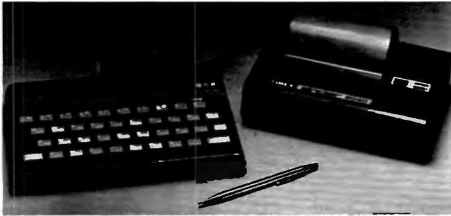
The Timex Sinclair 2000 is the first computer with 48K memory for under $200. Production models will have a topside cartridge slot for plug-in software. At right is the new thermal printer, which works with both the T/S 2000 and T/S 1000.
