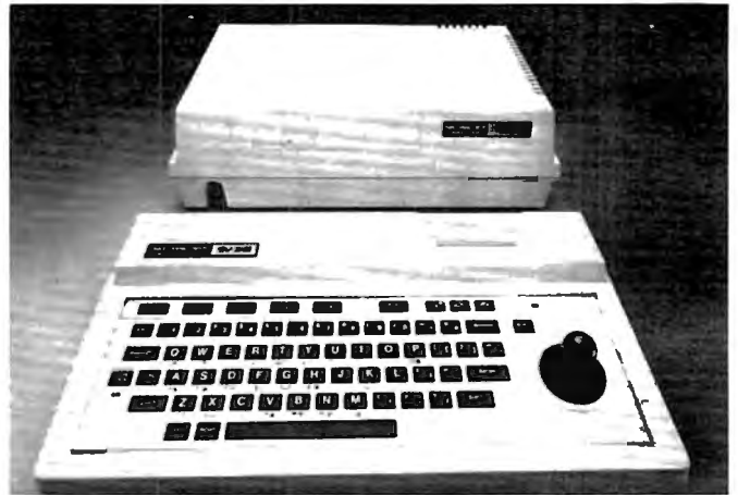
Spectra Video's new SV-318 computer and the optional Super Expander. Note the computer's topside slot, which accepts a $49.95 adapter for Colecovision game machine cartridges. Other adapters may also be available.
