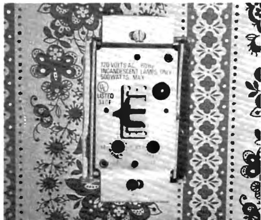
Photo 2: The wall switch module replaces the standard wall light switch. As with all the remote modules, it can be locally activated without the command console.
