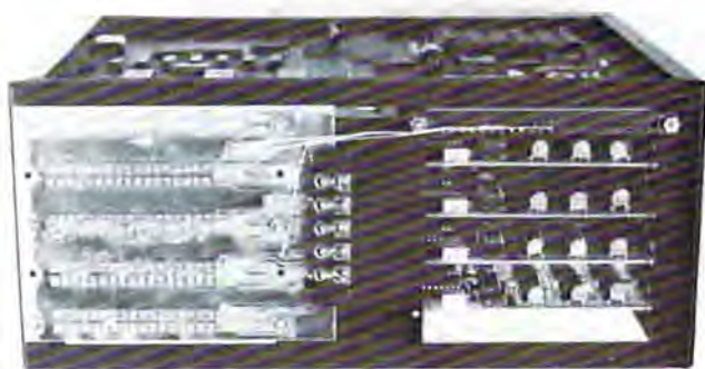
FIG. 1 KIM-1 INSTALLED IN A MICRO TECHNOLOGY UNLIMITED MOTHERBOARD/CARD FILE
