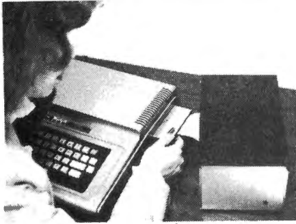
1. Here is Jeri plugging The Solution into the CoCo. Then she will move the main case up close to the CoCo. The cable is kept short to prevent noise and interference. The disk controller can be plugged into the side slot. The power supply plugs into a socket on the back of the case. All wires for the internal boards exit out the back of the case.
