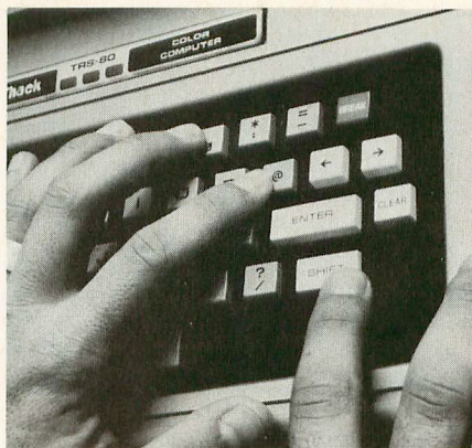
Photo 5. Press the SHIFT and @ keys at the same time to stop the video screen scrolling.
