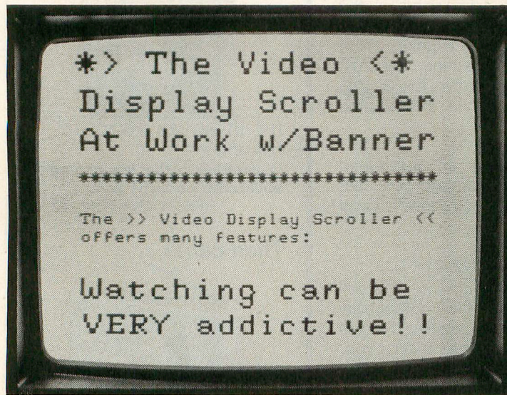
Photo 1. The Video Display Scroller in action. Banners stay in place, but text continuously scrolls by and repeats.
