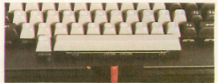
Micronix keyboard (bottom photo) with added red plastic support, and installed (top photo).
