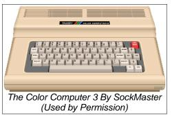
The CoCo 1 was an 8/16 bit computer running at 0.89/1.78 MHz. The text screen was 32 letters by 16 lines in uppercase. Graphics resolution was 256x192x2 although owners quickly found that color artifacting produced by the composite video output could increase the color count by one or two orders of
