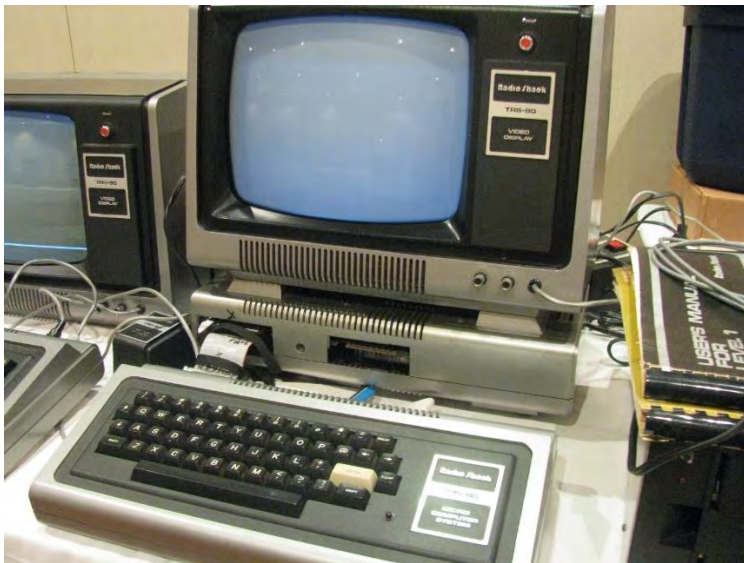
Radio Shack added the expansion port to the Model 1. This allowed more RAM and connectivity to external devices such as floppy drives, printers and cassette recorders. More information about this interface here: http://www.trs-80.org/radio-shack-expansion-interface/
