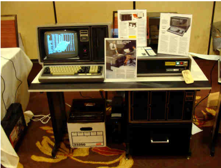
This desk is a recreation of an ad for the Model II (2) The desk holds three 8" floppy disk drives http://oldcomputers.net/pics/TRS-80-II_table.JPG
