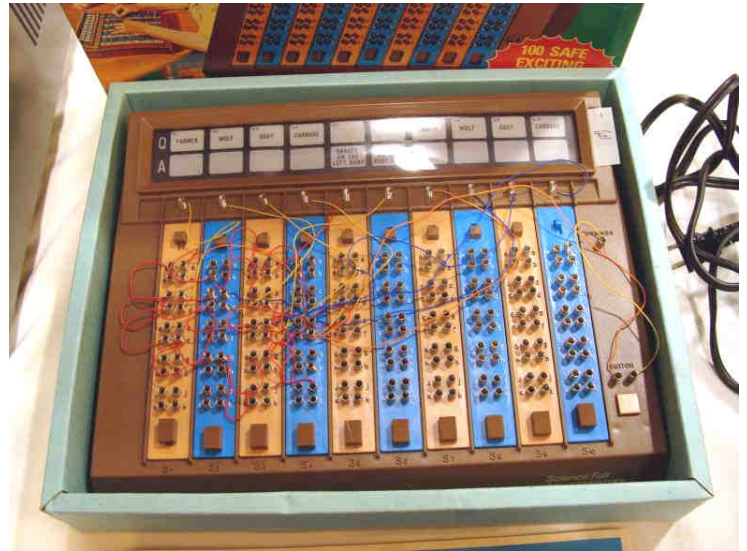
Ladder Logic Circuit each toggle switch has 5 normally open and 5 normally closed contacts. Uses incandescent lamps for output.
