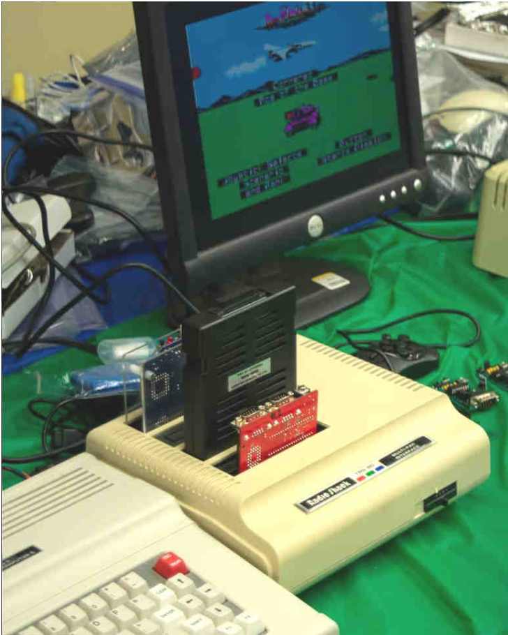
Multi-Pak Interface (MPI) This is a way to add more I/O Newer Multi-Pak designs offer more slots or I/O
