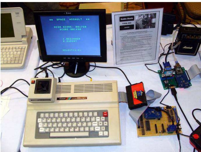
VGA CoCo+ Cartridge Slot-to-VGA Prototype Get CoCo 3 graphics on a CoCo 1 or CoCo 2 By: Peter Bartlett of Bartlett Labs http://bartlettlabs.com/
