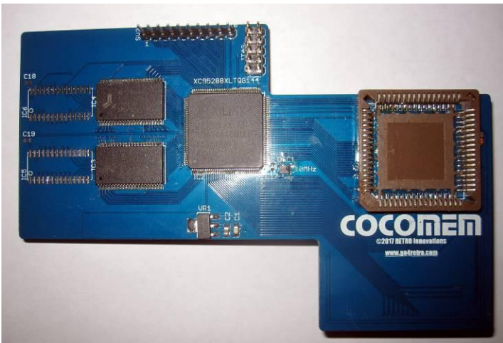
Product Name: CocoMEM Description: 2Megabyte static RAM upgrade that plugs into the GIME socket. No soldering and no clip leads required. Current state: In development
