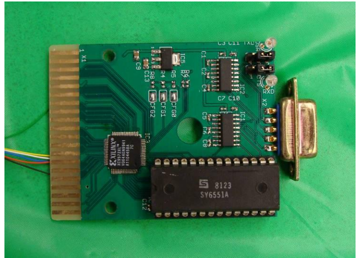
Product Name: CocoLINK Description: Tandy RS232 Pak functionality with additional speeds (38.4kbps, 57.6kbps, 115.2kbps, 230.4kbps) Current State: Design complete, waiting for sufficient community interest to start production.
