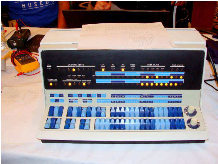
This is a DEC PDP panel. You can use it to enter, examine, and single-step your code.
