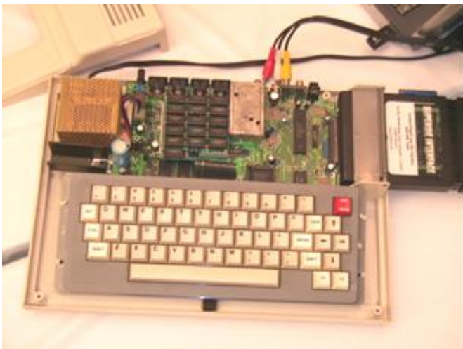
Yet another CoCo with a RAM expansion module and the SuperIDE Interface.
