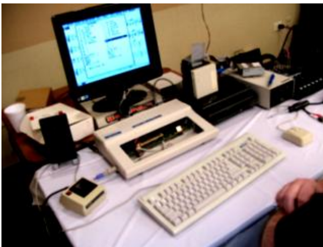
The CoCo setup used a PS/2 keyboard plus other interfacing hardware for the MIDI setup.
