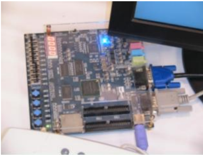
A close up of the Altera DE1 board used for the Color Computer Emulator.
