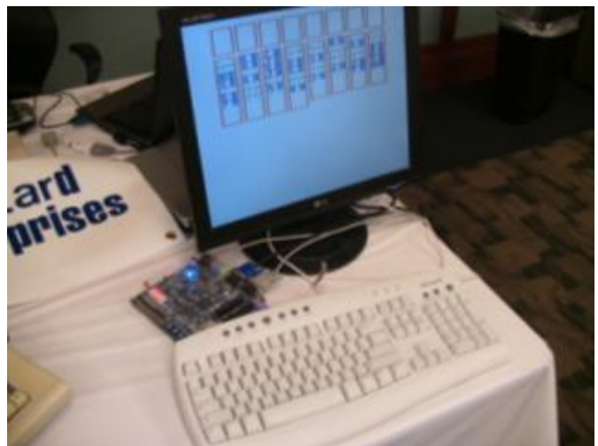
A complete shot of the FPGA Color Computer using a VGA monitor and PS/2 keyboard.
