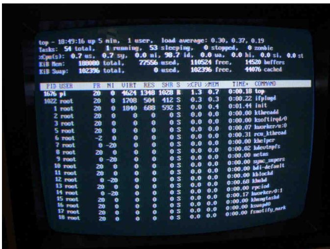
Composite video on a Raspberry Pi showing top
