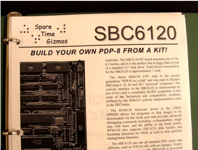
Single board computer SBC6120, a PDP-8 emulator
