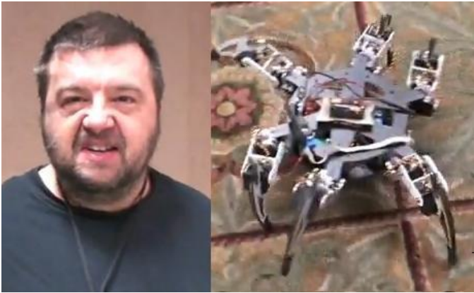
Roy Justus was showing off a six legged, 18-servo hexapod robot. The creature was controlled from his Color Computer 3 using Bluetooth wireless to communicate with the hexapod.
