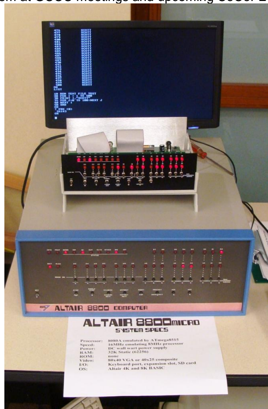
Mini Altair Clone Kit on Top of an Original Altair Computer
