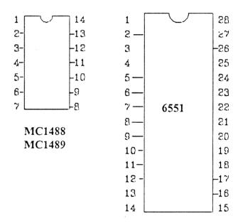
Now, piggyback the 1488 to the original on the board and do the same with the 1489. Solder only the pins you left pointing down at this time.
