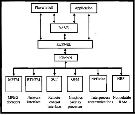
DAVID includes a SCF (sequential Character File Manager that is used to communicate with remote control devices. A user control task, communicating via the SCF, could sense the rewind command from the user, and via PIPEMan, start the process to rewind the program. A network control task would use the bidirectional capabilities of the RTNFM and the network to send the command to the programming provider.
