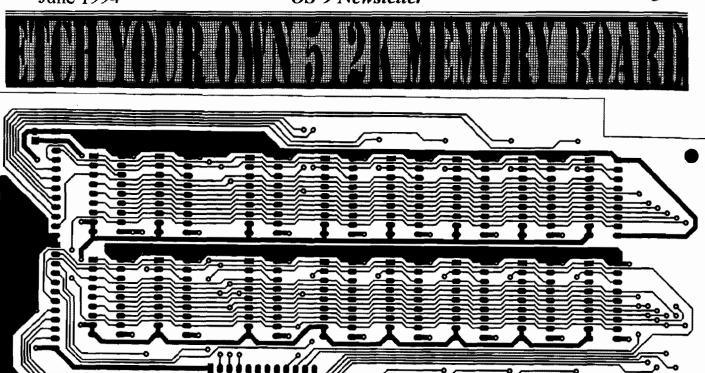
One of the reasons I bought my CoCo-3 was the price. Both hardware and software were being closed out at ridiculously low prices. The trouble was, the upgrade to 512K was still just as expensive as ever. Well, being a long-time hobbyist, and having access to a Printed Circuit Board design CAD system, I figured I would MAKE MY OWN BOARD. It would be single-sided, avoiding the expense of through-hole plating, and putting the 512K upgrade within almost anyone's read.
