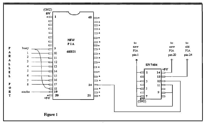
Press the 40 pin IC socket over the top of IC4 and solder socket pins 1, 20, 21 - 23 and 25 - 40 to the corresponding pins on IC4. Solder a 4 inch length of thin hookup wire to socket pin 24.
