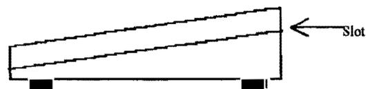
The dimensions are 5 inches long, 3/4 inch wide, 1-1/2 inch high at one end and 3/4 inch high at the other end. Cut a 1/2 inch slot, 1/16 inch wide and 1/2 inch from the top angle cut. The blocks will press fit on the end of the keyboard and can be finished with varnish, varathane or paint. With the extra wires, you can add an LED Power On light and even a reset switch.
