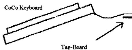
4. Use *Elmer's Glue* to attach a piece of tag-board or thin card-board (such as used to package electronic components) under the mylar keyboard cable so that the combined thickness of the mylar cable and the tag-board will provide a solid contact when inserted into the other *Kel-AM* Connector.
