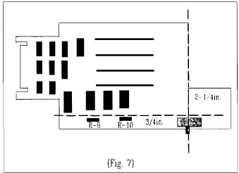
I trimmed 3/4 of an inch off the side of the circuit board. The switch was not really necessary since I would not need to switch it from slot 4 (I don't use ROM-PAKS). I cut off the 2-1/4 inch square part of the circuit board that contained the voltage regulator (with the big heat sink). Then I only had to remount R-9 and R-10
