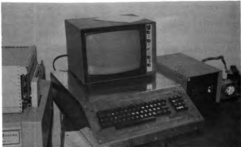
Photo 3. The LNW microcomputer in one of the author's homemade sheetmetal cases.
