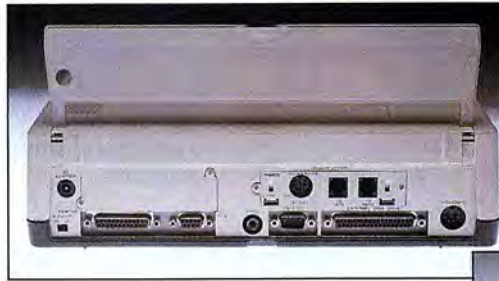
Metal cover on the back of the 1400 LT conceals an undocumented expansion slot.
