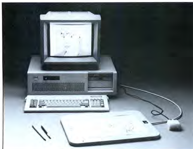
The Easy! PC tablet comes with an interface card that includes one port for the tablet and one for a serial device.
