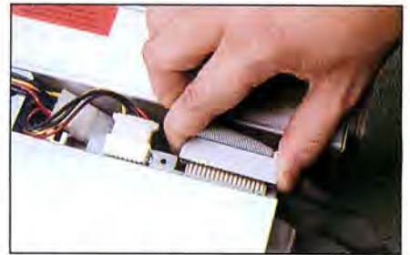
Slide the new drive into the empty drive bay above Drive B. Attach the power connector and the drive controller cable; be sure to invert the drive cable before connecting.
