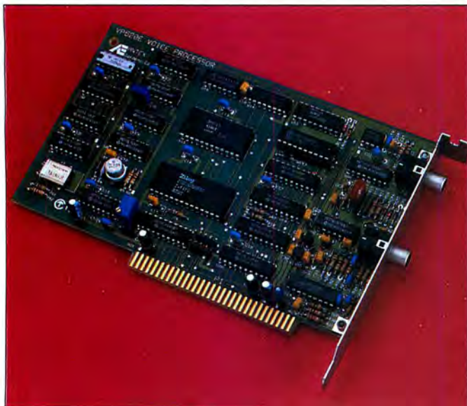
VP620E voice processor digitizes audio signals for recording or random playback on computer disks.
