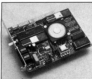
Zoom/Modem provides an on-board speaker with volume control and an audio jack.
