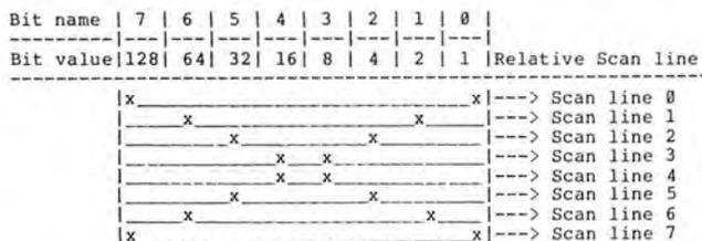
Figure 2. A breakdown of a video cell by scan code and bit position.
