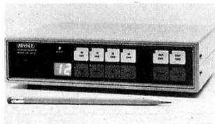
Keydex Buffer and Printer Sharer can connect up to four computers and two parallel printers.
