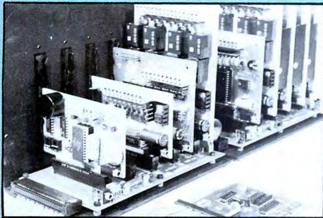
An A-BUS system with two Motherboards
