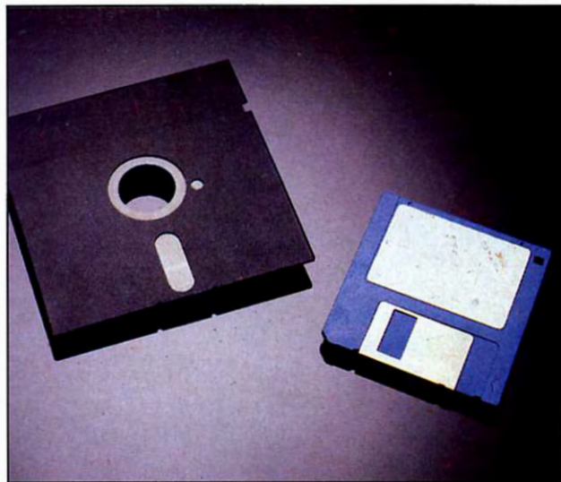
According to predictions, microfloppies will become standard replacing the 5¼-inch disks by 1989.
