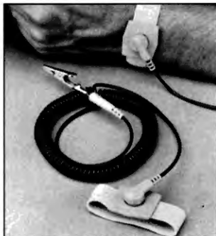
A wrist strap to prevent static charges.
