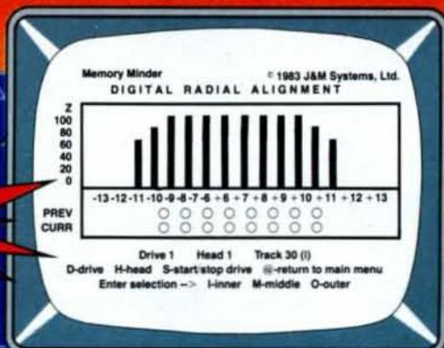
Use the MM Radial Alignment Test to check the head alignment of your drives. No need for an oscilloscope or other expensive test equipment!
