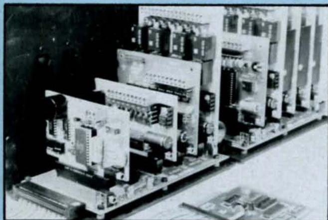
An A-BUS system with two Motherboards
