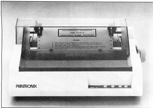
The Printronic P1013 can print IBM block graphics in draft or letter-quality modes.
