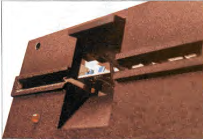
Photo 1. The potentiometer and small brass adjusting screw seen through the disk drive latch.
