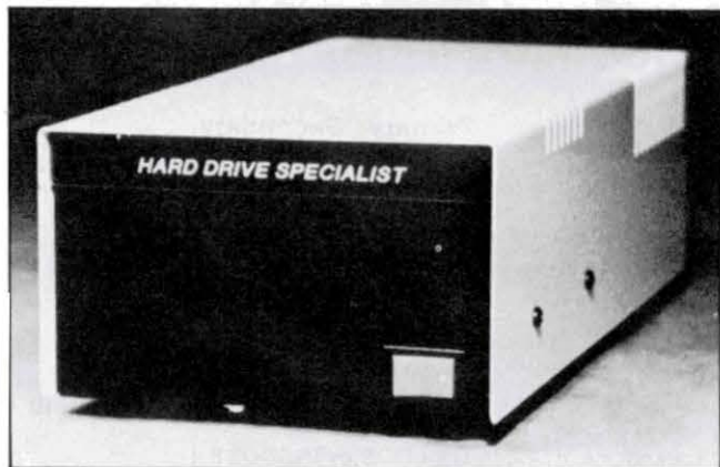
The Hard Drive Specialist Multiplexer for up to four computers.
