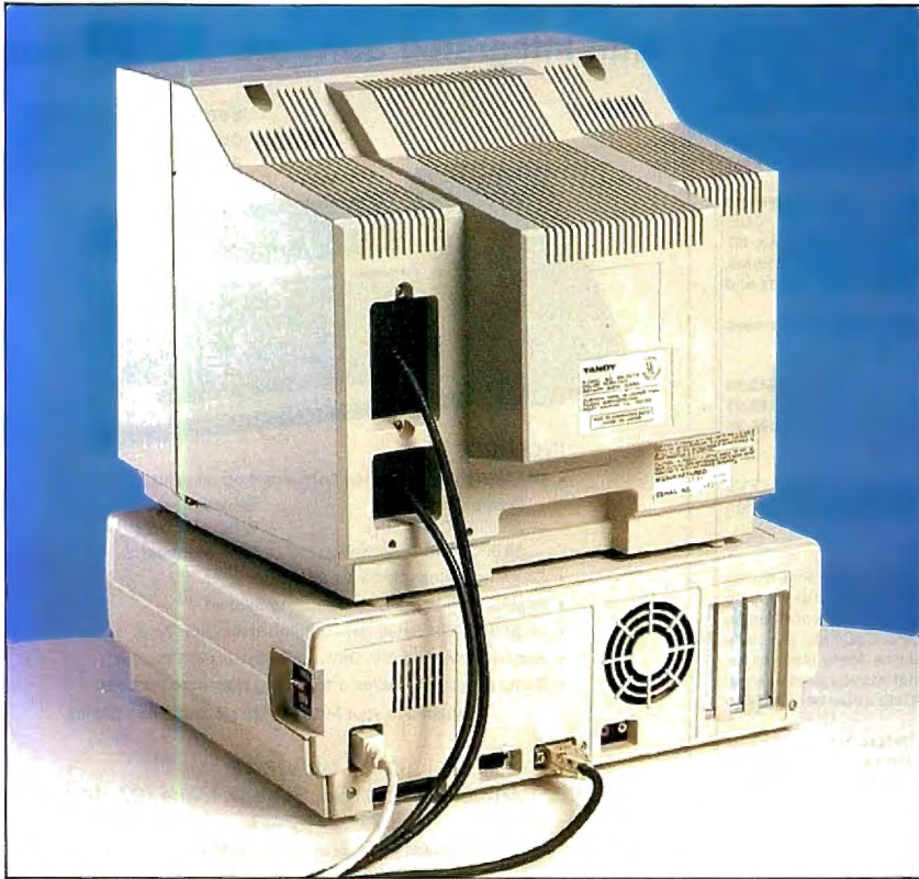
Photo 2. Rear view of Tandy 1000 (showing lighted power switch on side). The printer port edge connector is under the power plug on the left. To its right, along the bottom, are user ports for a light pen, RGB monitor, and the video and audio signals. To the right of the fan exhaust are covered openings for the three expansion slots.
