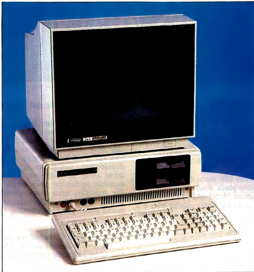
Photo 1. The 384K Tandy 1000 used in this review with CM-2 color monitor. Model 2000 styling includes the 2000's keyboard. The horizontal slimline drives are to the right. Along the bottom recess, from left to right, are the orange reset button, the keyboard plug, two joystick ports, and a ventilation grille.
