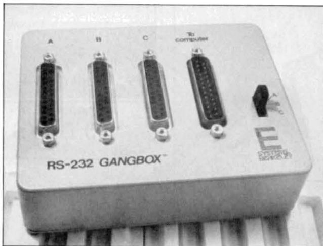
Gangbox expands your RS-232 port to accept three peripherals.
