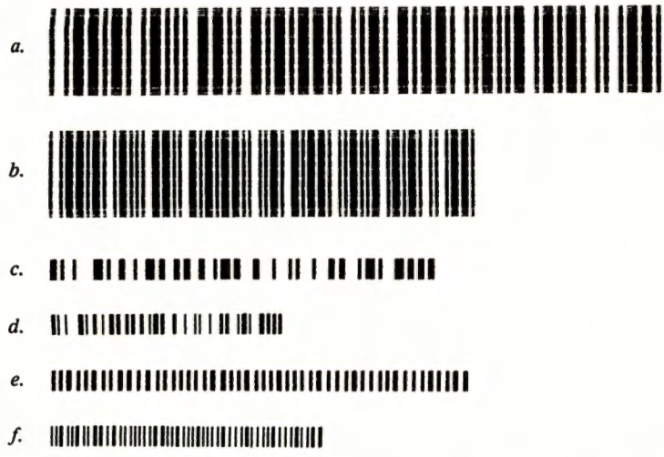
Figure 1. Comparing the density of different bar codes. Each code translates to read "80 Micro." (a.) A conventional-density code, 3 of 9, in standard format; (b.) 3 of 9 in compressed format; (c.) A high-density code, Code 128, in standard format; (d.) Code 128 in compressed format; (e.) Dense Tandycode in standard format; (f.) Tandycode in compressed format.
